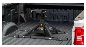
Even with its robust 20,000-lb. rating, CrossWing is much lighter weight than traditional 5th wheel hitches, with the main body only weighing 60 lbs.
